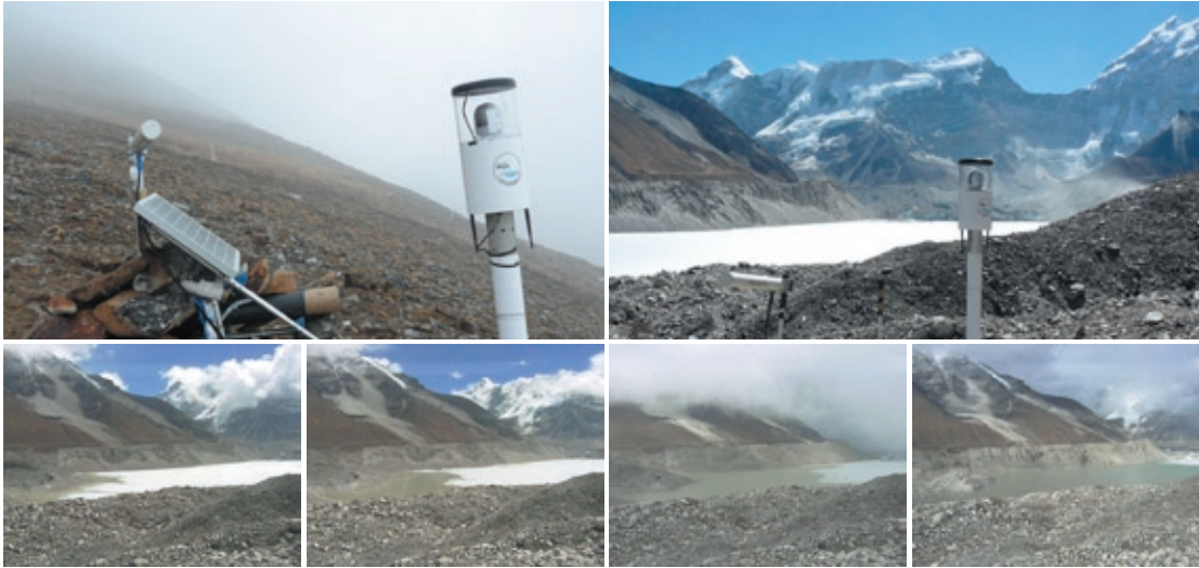
Field servers that Professor Fukui's research team has installed around Imja Glacial Lake (above). Images of Imja Glacial Lake photographed by the field servers between May 9 and 12, 2008. The ice on the surface is clearly melting (from left to right).
