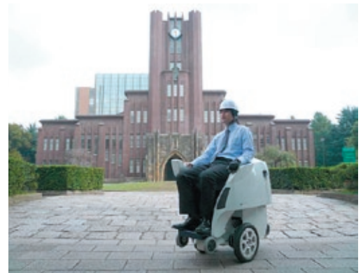
A researcher rides a Personal Mobility Unit, specially built for outdoor use, on the University of Tokyo grounds. The Unit can be operated without the use of the hands.
