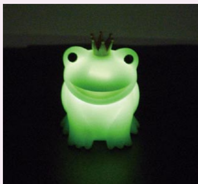
A frog-shaped lamp lights up when placed on electricity-conducting CNT paper.
