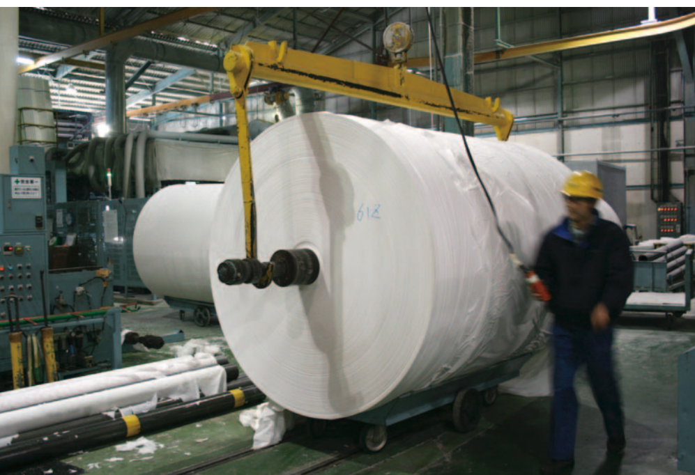
A giant roll of toilet paper. The paper is turned into product-size rolls and then cut.
