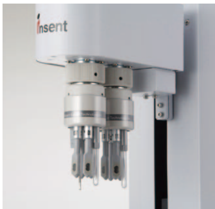
Taste sensors tipped with artificial taste cells.
