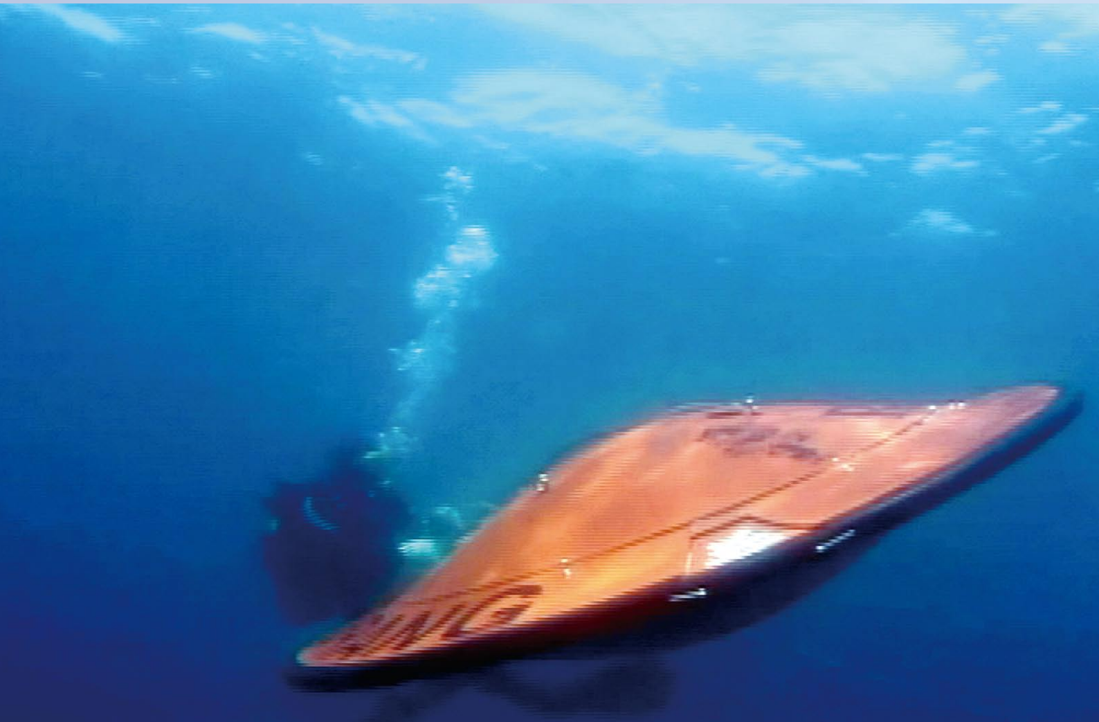
A submersible disk-shaped probe, dubbed the Boomerang, glides through the ocean. Photo Kyushu University
