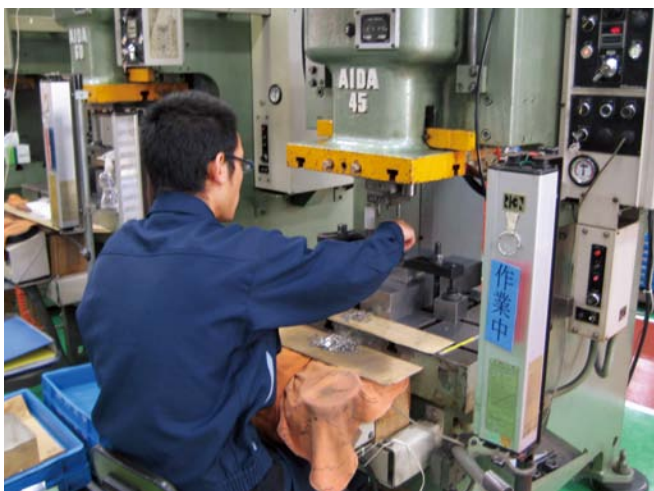
Kamite Co., founded in 1988, produces parts of machines such as cameras, printers and TVs. An employee makes parts using a 45-ton press in the factory.
