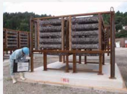
A shelf-like standard JF Shell Nurse installation (fish-breeding type (2.2 model))
