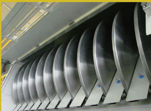
The CD Dryer model with 12 disks arranged inside the unit.
