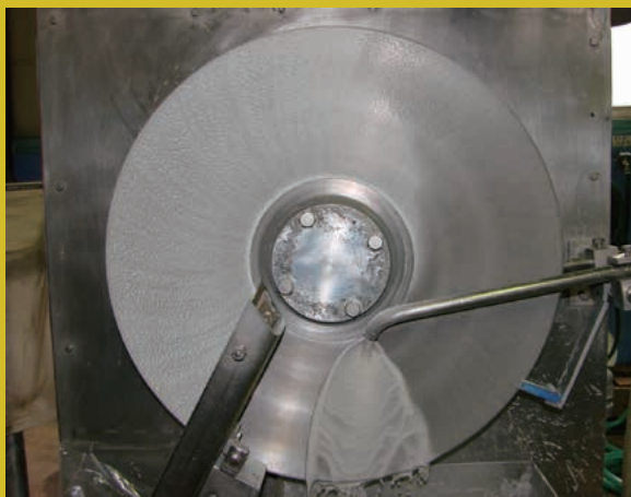
The process of pouring the target liquid onto the rotating disk.
