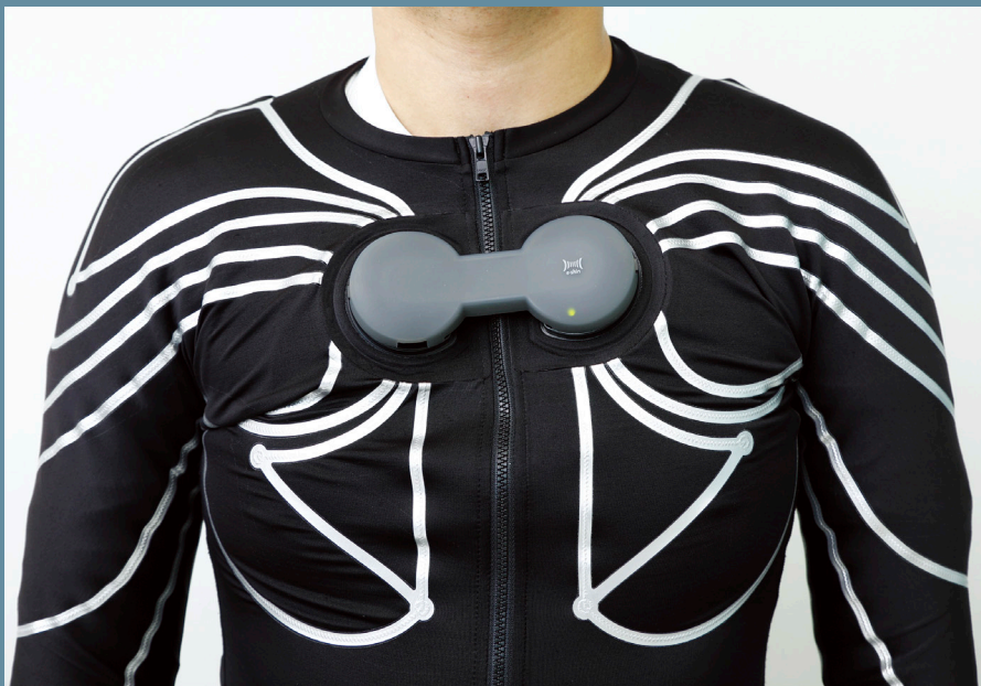
This elastic e-skin shirt has fourteen sensors and an “e-skin Hub” that collects and stores information
