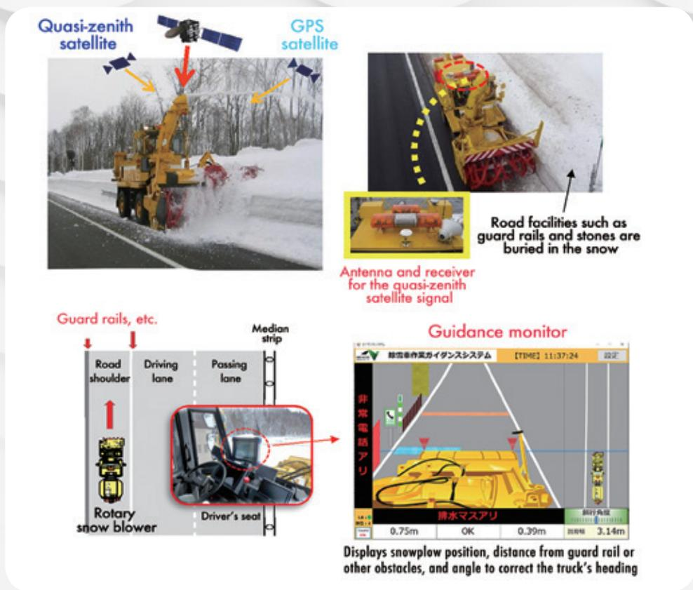
“The driver’s seat monitor displays driving lane overlap and where to point the truck or how to correct its trajectory in order to avoid contact with the guard rail. This enables even less experienced operators to plow safely and surely,” says Nakatani.
