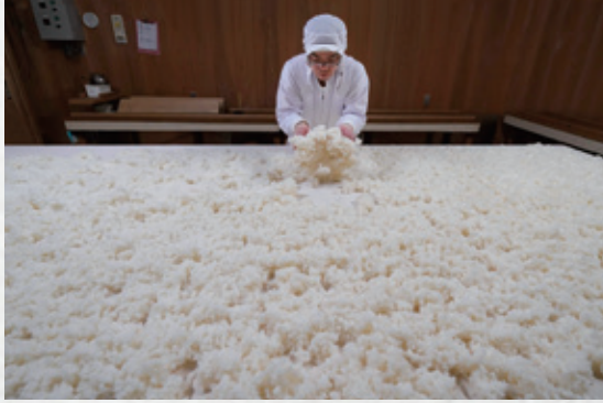
■ In a process known as tokomomi , a brewer kneads koji spores into a bed of steamed rice Courtesy of Daishichi Sake Brewery Co., Ltd.
