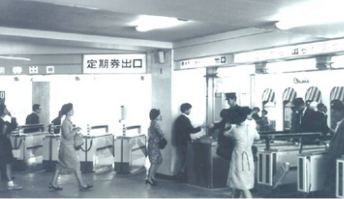
The world's first automated ticket gate system developed by Tateishi Electronics Co. (currently OMRON Corporation) was introduced in the Hankyu Railway at Kita-senri Station along the Hankyu Senri Line in 1967. Photo: Courtesy of OMRON SOCIAL SOLUTIONS CO., LTD.
