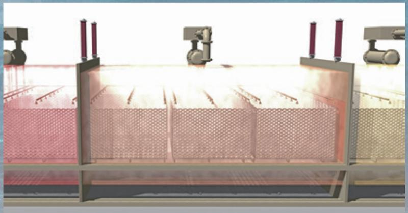
Each unit in the "continuous process" series of Urban Rig has a distinct temperature setting, enabling efficient extraction of light diesel oil and other products at different points along the line before cooling
