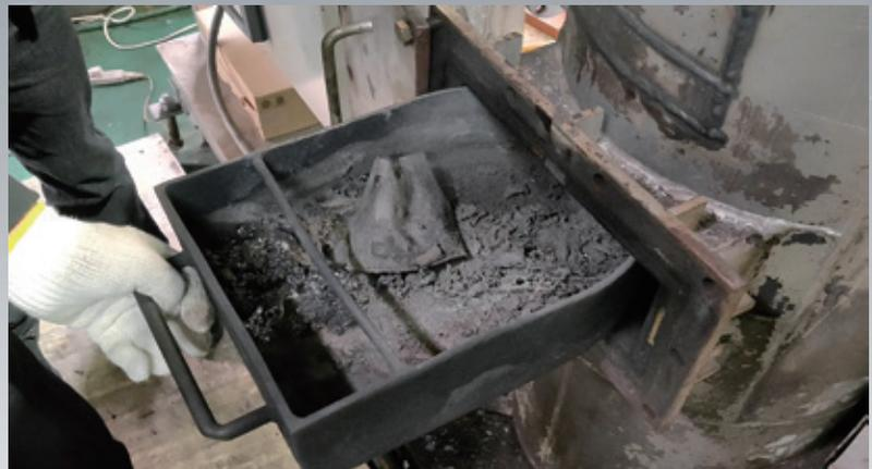
The carbonized ash (charcoal) recovered after processing with Urban Rig can be used as fuel
