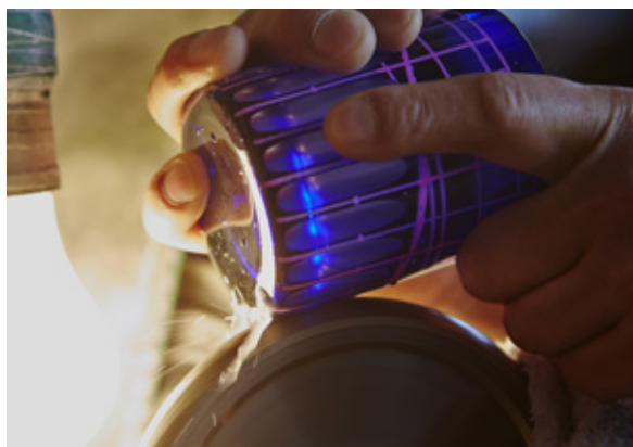
Patterns are cut into the glass using rotating grindstone tools Photo: Courtesy of the Edo Kiriko Cooperative Association
