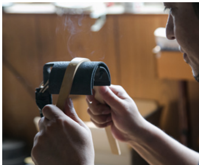
Bending bamboo over heat to form the product frame. Holes are drilled in the frame into which bamboo strands are inserted to assemble the product.
