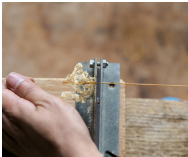
Stripping bamboo strands ( takehigo ) for the lattice work
