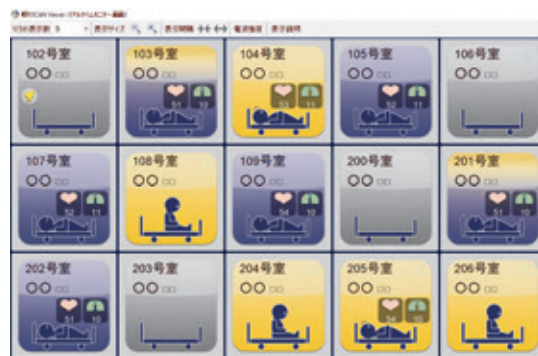
■ A visualization of patients’ heart rates, respiratory rates and states (sleeping, out of bed, etc.) is displayed in real time on the monitor
