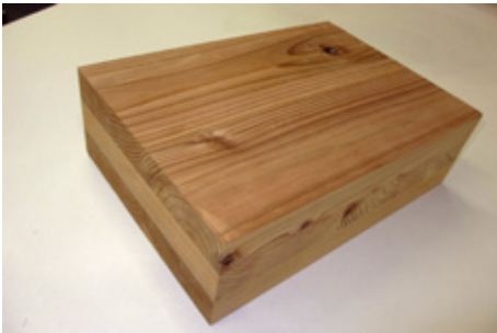
A block of Cross Laminated Timber (CLT)—planks of wood glued together in layers, with each layer oriented perpendicular to the previous
