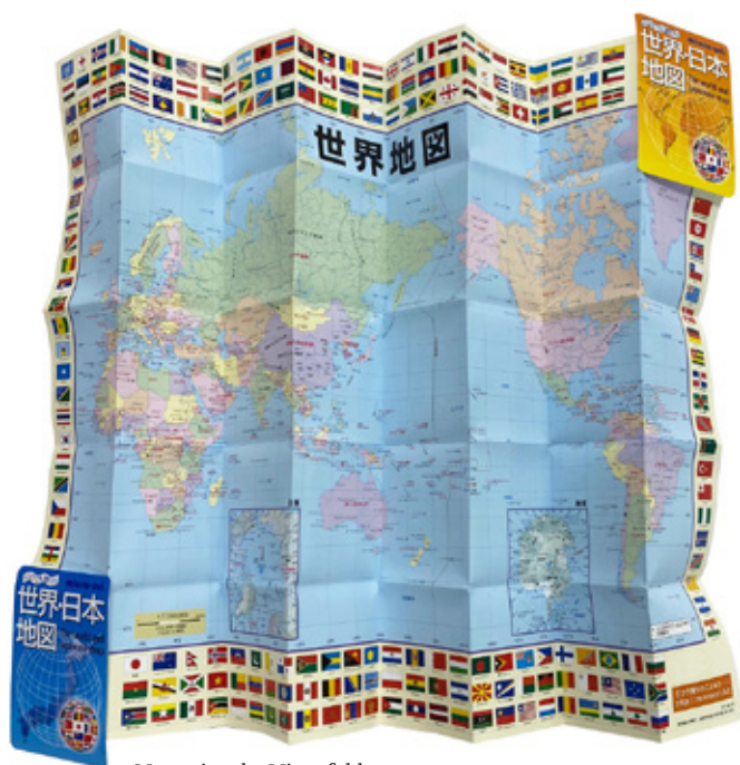
Map using the Miura fold Photo: Courtesy of Inoue General Print Co., Ltd.
