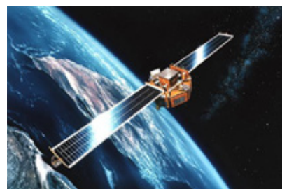
Space Flyer Unit (SFU), a satellite equipped with a planar structure made using the Miura fold Photo: Courtesy of JAXA
