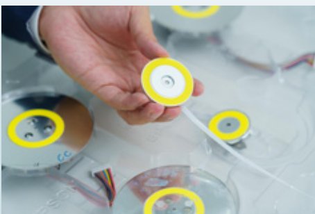
Yellow phosphor applied to disks. When illuminated by a blue laser light source, the disk reflects yellow light
