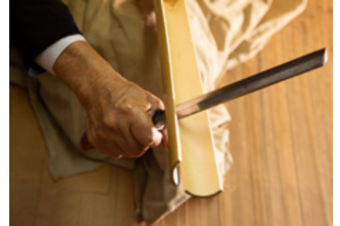
Creating bamboo strands ( takehigo ) by splitting the bamboo
