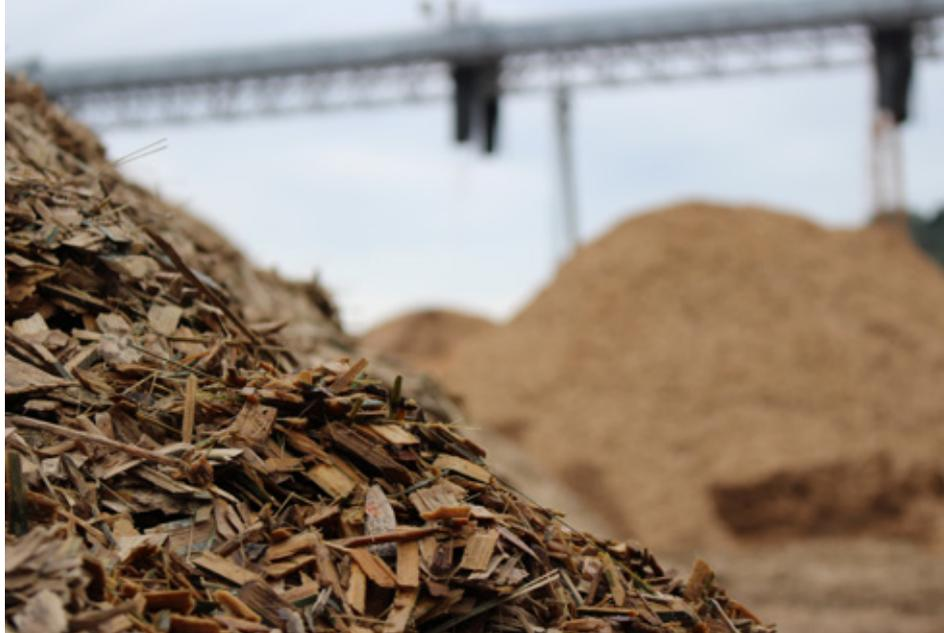
Bamboo chips, the raw material for bamboo papermaking
