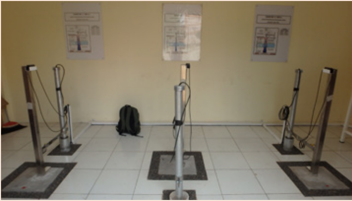
Monitoring wells installed in northern Jakarta to observe the state of land subsidence
