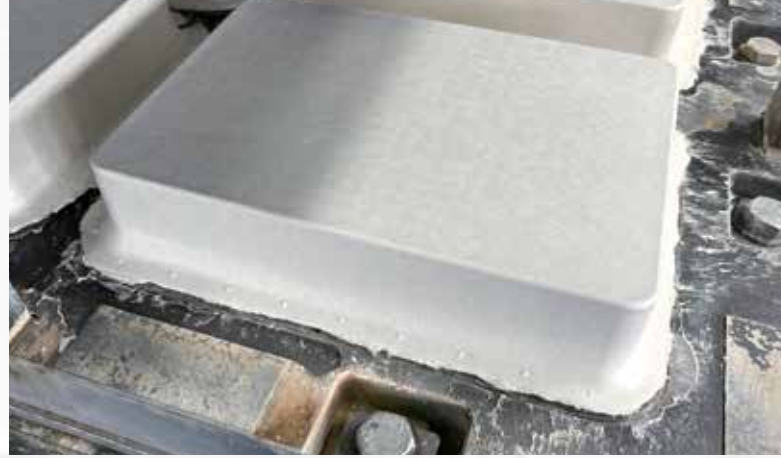
The smooth curves and surfaces of kome-kami BOX are finished by applying pressure at high temperatures,
